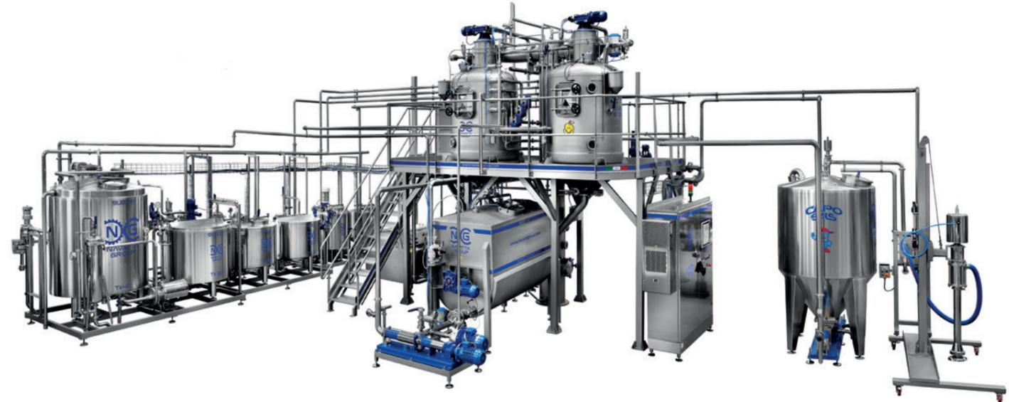
Tomato mix, ketchup and jam processing line with ingredient feeding and mixing system pre-built and FAT tested before shipping
