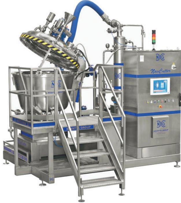
Under vacuum cutter with the function of crushing/mixing/cooking of products, combining them with vacuum and thermal processes. Ideal for high viscosity formulated products like jams, salted and sweet creams, sauces, jellies, yogurts
