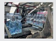
Shrink wrapper Ocme Vega S60/2 for packaging with thermo retractable
